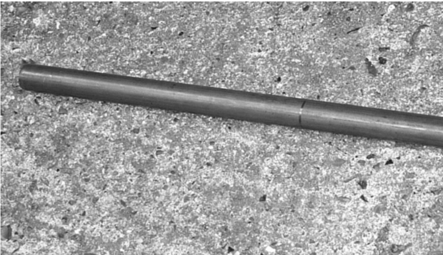
fig 99: pencil mark the pipe where you want to make a bend
