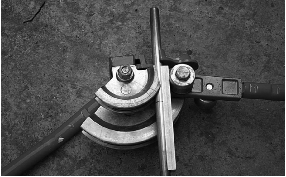
fig 100: place the pipe in the hand benders, slide in the bending guide and align the pencil mark
