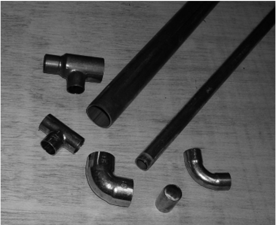
fig 66: copper tubing with copper end-feed solder fittings
