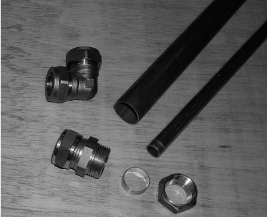
fig 67: copper tubing with brass compression fittings
