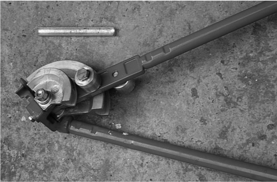
fig 98: hand benders with metal guide
