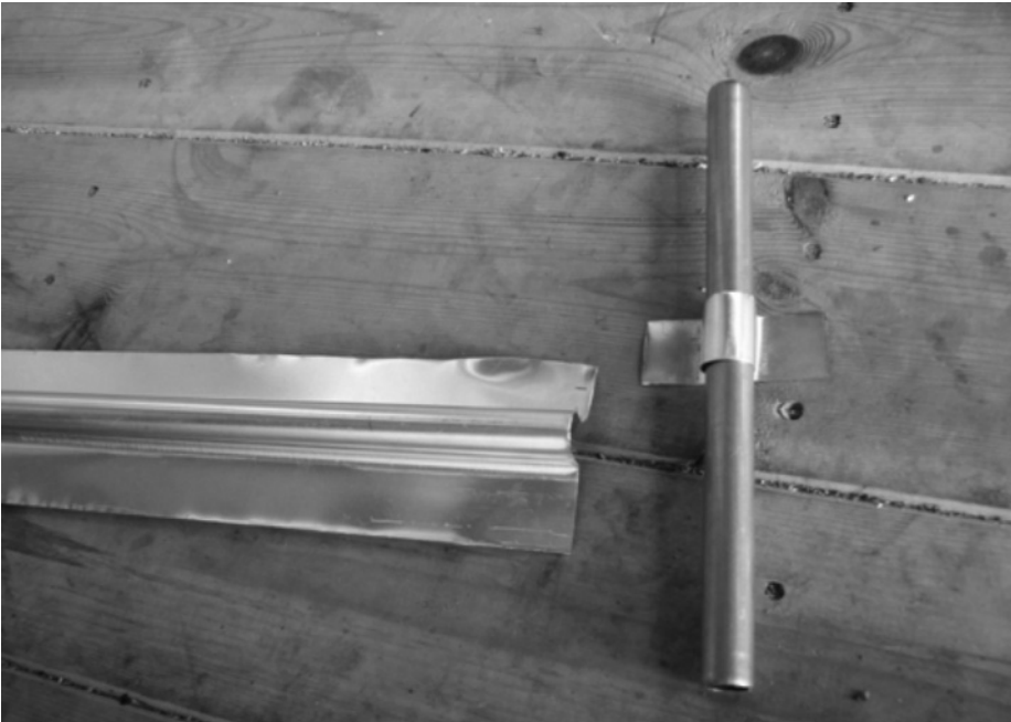
fig 173: use left over aluminium to make pipe clips
