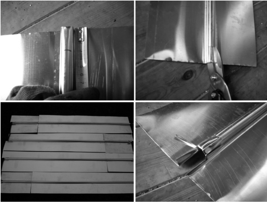
fig 161: preparing the spreader plates
