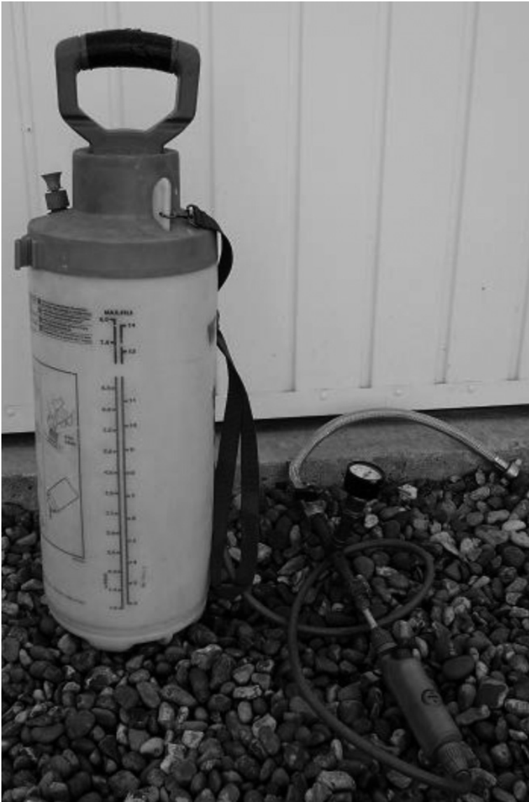
fig 74: A good garden sprayer is often designed to pressurise fluid up to 3 bar so makes a handy tool for the job of filling a pressurised solar thermal system
