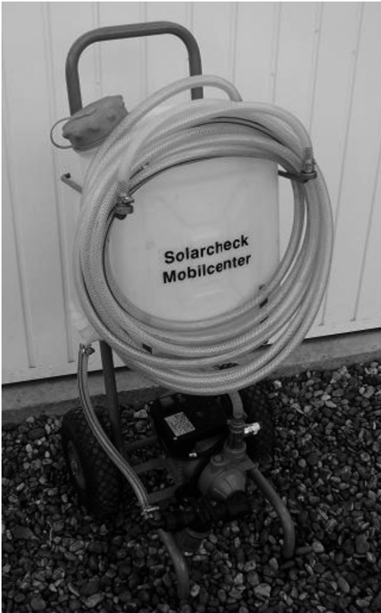
fig 76: filling and commissioning machine
