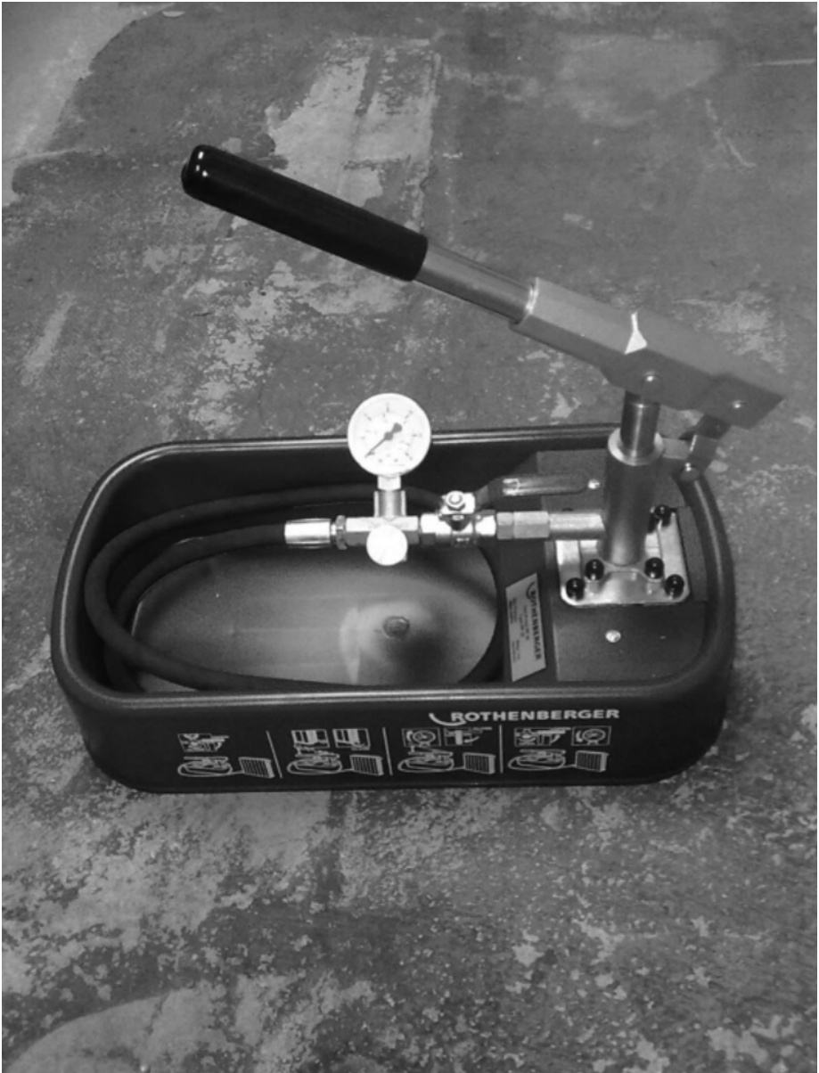
fig 75: pipework pressure testing pump
