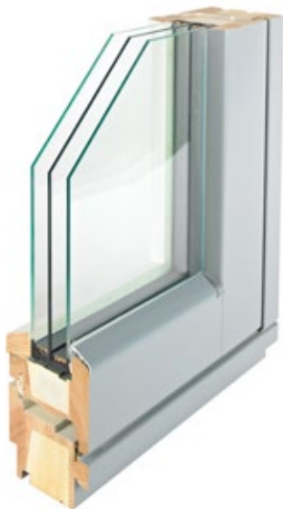
Figure 7.4 Triple glazed low emissivity gas filled glazing with insulated spacers in insulated timber frame, giving a whole window U value of 0.68 W/m²K (Green Building Store)
