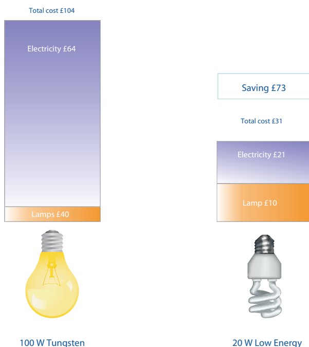
Figure 12.2 Even at a cost of £10 the compact fluorescent lamp saves seven times its cost over its life
