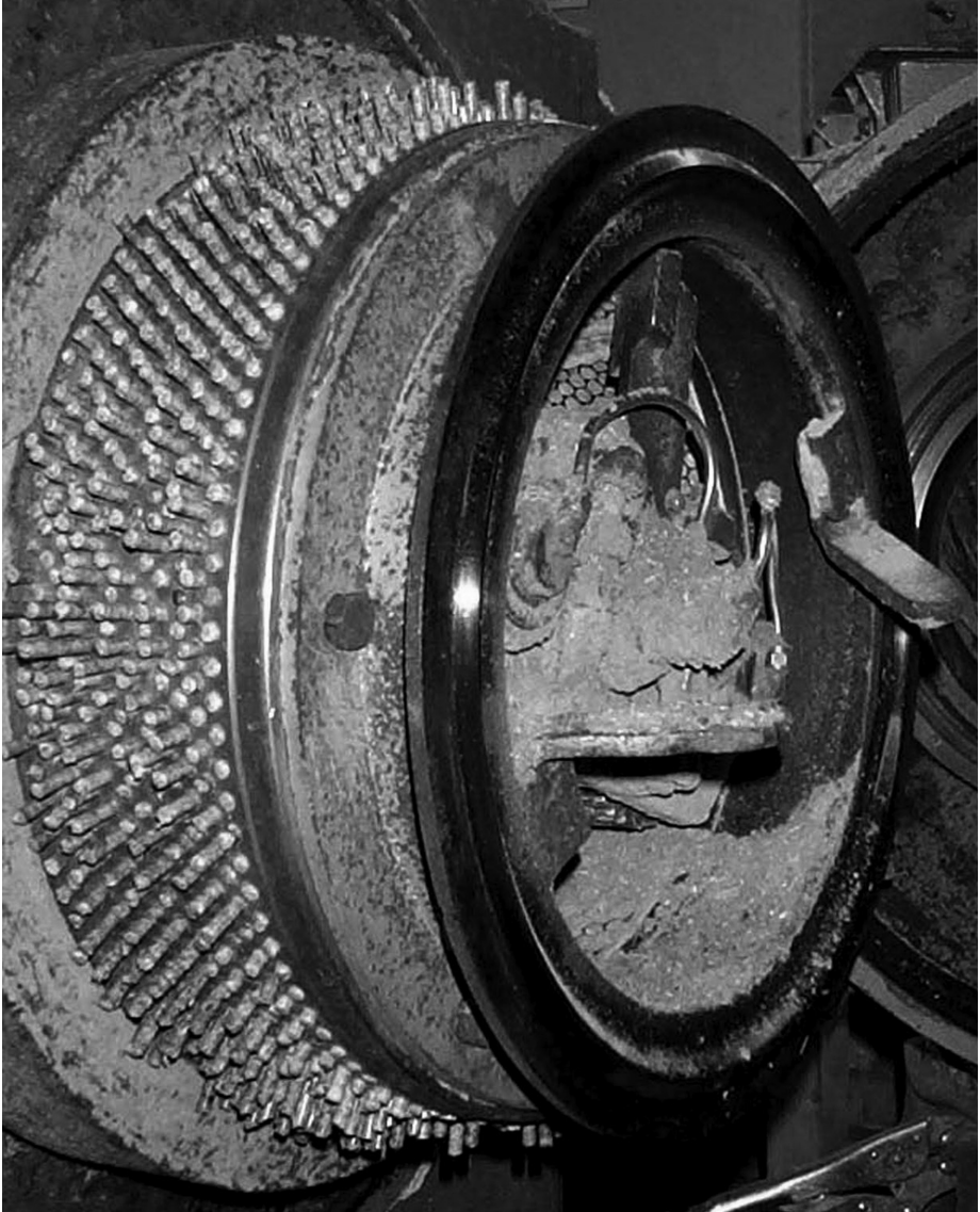
fig 29: a wood pellet machine with the cover removed, showing pellet die with extruded pellets
