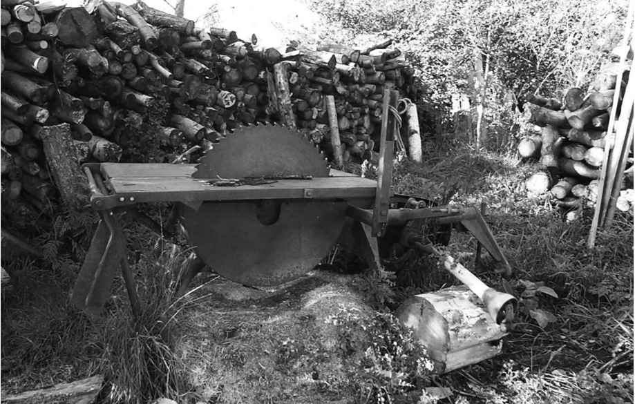
fig 7: tractor driven saw bench (guard removed for clarity)
