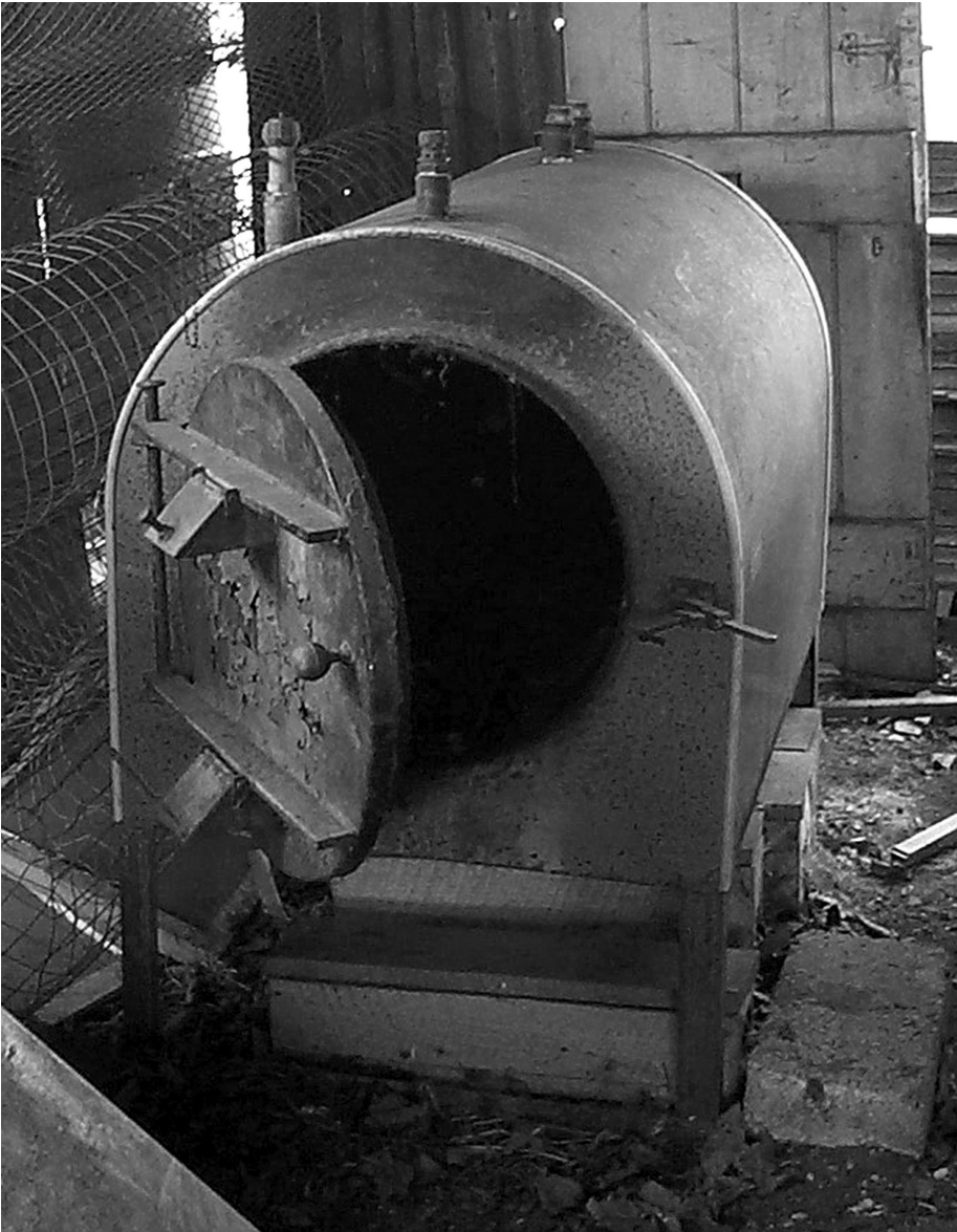
fig 34: basic batch boiler
