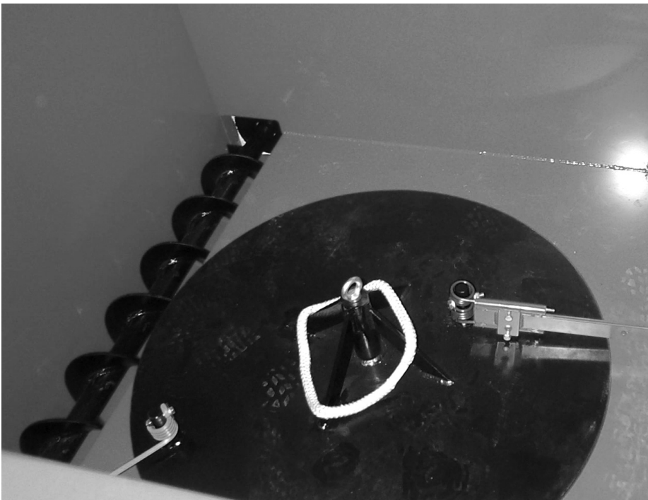
fig 30: feed auger and agitator
