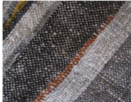
Plain weave showing warp & weft threads.
