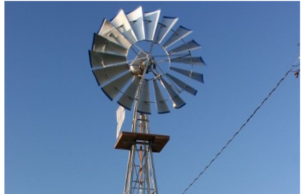
A wind pump – a way of getting water to where you want it without using electricity.
