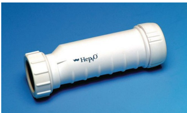
A HepVO valve is a self-sealing waste valve - the easiest way to convert a flush urinal to a waterless one (apart from no trap at all). It may be too flimsy for a heavily-used urinal.
