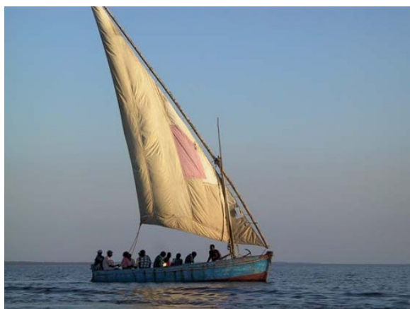
Triangular lateen rig on an Arab dhow.
