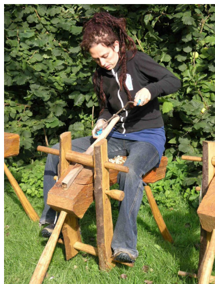
Using a shave horse and draw knife to cut a peg roughly to size.
