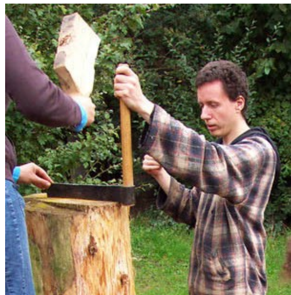
Splitting a log with a froe and a wooden mallet.
