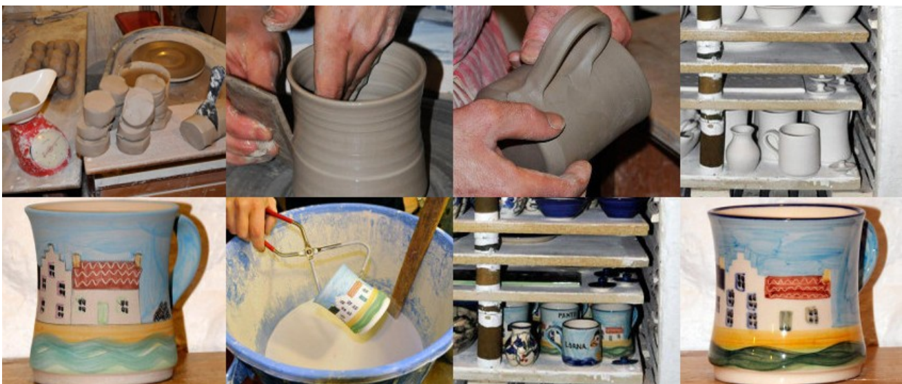
From clay to mug: cutting and weighing clay; throwing; adding a handle; bisque firing; decorating; glazing; glaze firing; finished mug.
