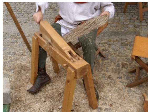
Flax Brake – traditional method of separating the fibres from the stem by hand.
