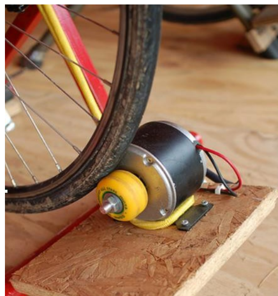
Turning a generator via a friction roller.
