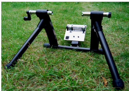
Pedal-powered generator stand onto which you fix your bike to generate electricity.
