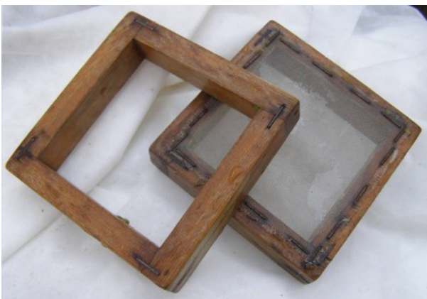
A simple, home-made mould and deckle.
