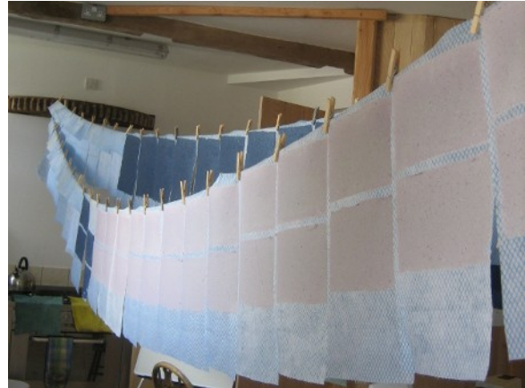
Paper hanging to dry, still attached to felts.
