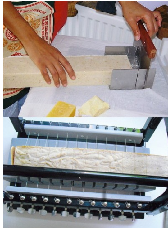
Two ways of cutting the finished soap into bars.
