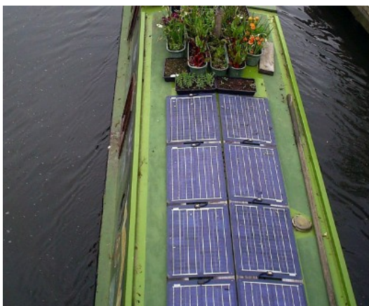
Solar panels on the roof of a narrowboat – quieter and cleaner than a diesel generator.
