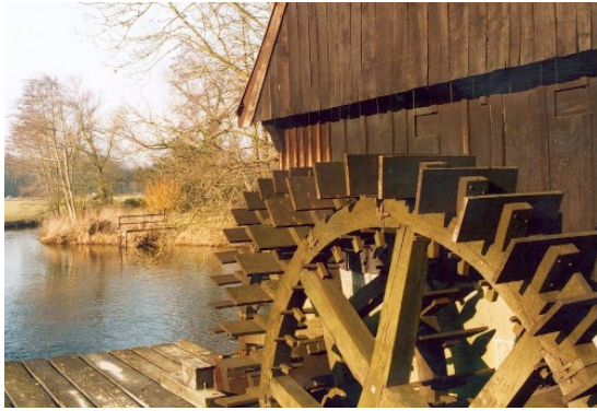
Old-style watermill, originally used for milling grain, can be used to generate electricity.
