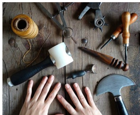
A leatherworker's tools. Top, l-r: waxed thread and needle, wing divider, hole punch, awls. Middle, l-r: mallet, swivel knife for carving, edge slicker. Bottom, l-r: skilled hands and leather cutting knife.
