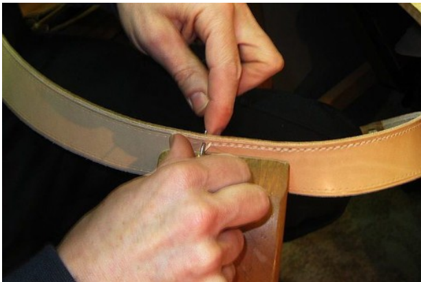
Sewing leather: saddle stitch with two needles, held in place by a stitching pony.
