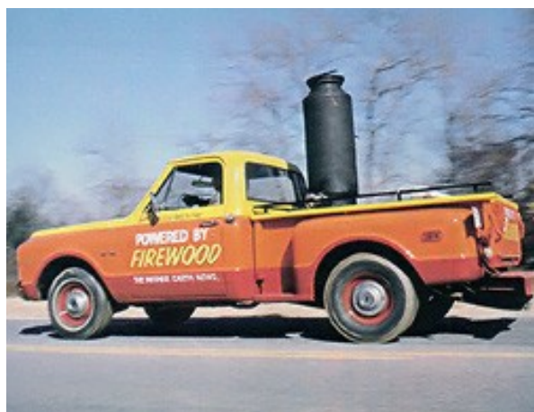
Pickup with gasifier tank on the back. It's filled with wood scraps and the gas is piped to the engine.
