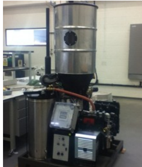
10kW combined downdraft biomass gasifier with engine and generator.
