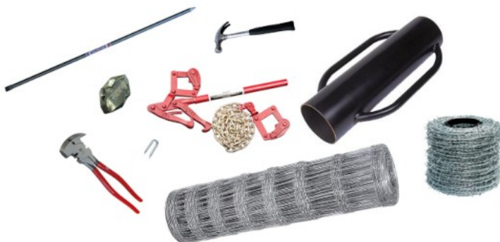
Tools and equipment that you'll need for a standard sheep fence: clockwise from top left – crowbar, hammer, post driver, roll of barbed wire, roll of sheep netting, gripple wire joiner (optional), wire strainer, staple.
