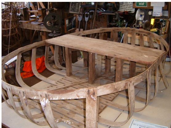
Building a coracle in a workshop; the gunwale is the strip around the top, to which all the other strips and the seat are connected.
