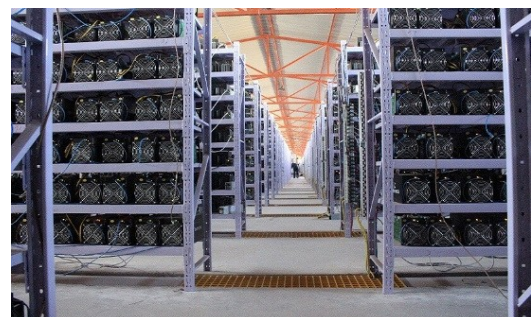
Huge computer banks do the puzzle-solving involved in 'proof-of-work' algorithms used to generate Bitcoin. 'Proof-of-stake' algorithms use far less electricity.
