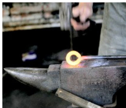
Blacksmith hammering and bending a heated rod on the face of an anvil.
