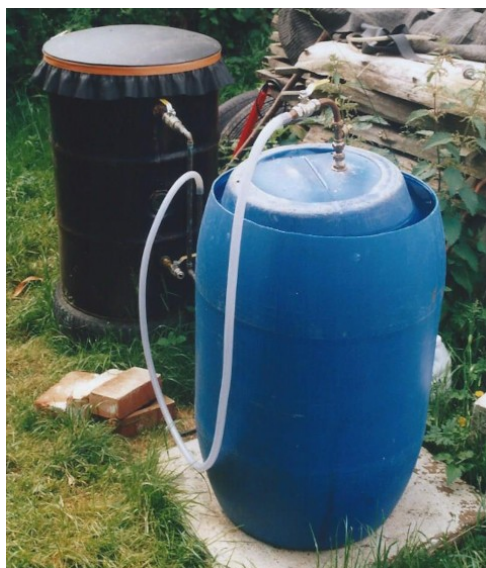
Small experimental biogas digester. Waste material is put into the oil drum; the neoprene cover rises when full of gas; the gas is tapped into a container (upside-down plastic drum with water seal) which rises as more gas enters. When full, gas can be tapped off and used via a little gas ring.
