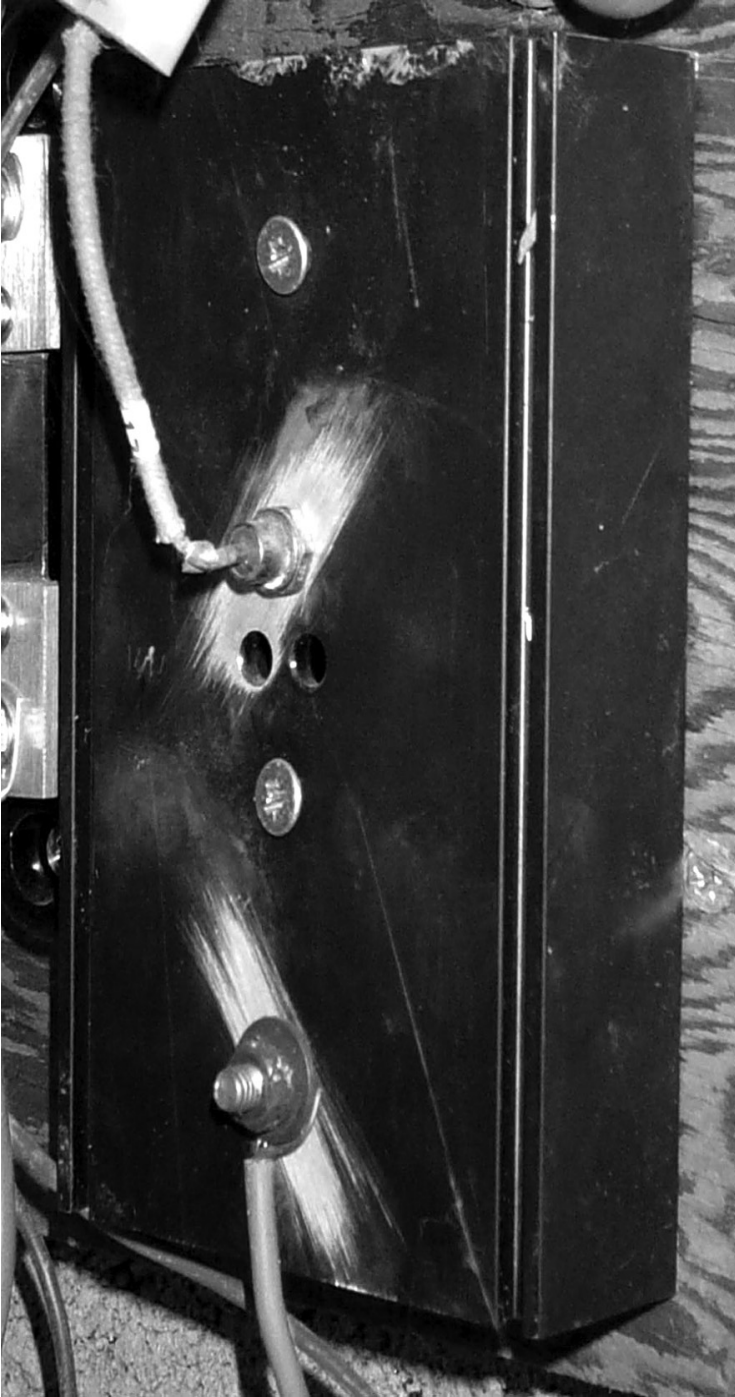
fig 59: blocking diode on anodised aluminium sheet
