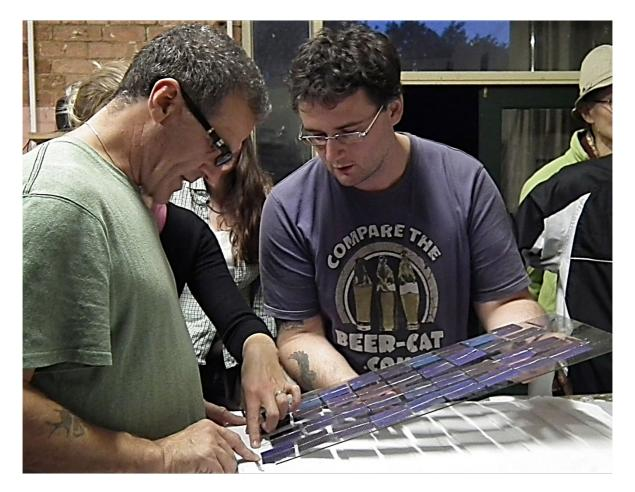
i. Lay all four strings face up on your sheet of glass, don't worry - the glass does not need to be cleaned at this stage. Ensure that when all four strings are connected in this way the cells are still alternate - the top connection on one cell must contact the bottom on the next cell.
