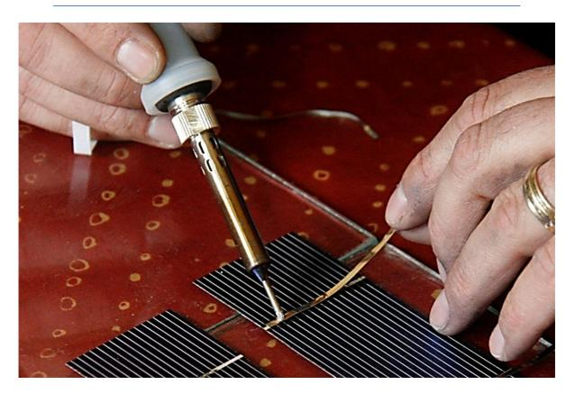
A soldering iron able to reach high temperatures is required to solder the ribbon to the solar cells. Most 'off-the-shelf' soldering irons available in DIY/hardware stores will not be suitable. The soldering iron should be at least 60 watts or able to be set at 450+°C. A bevelled soldering tip of about 3mm is also preferable.
