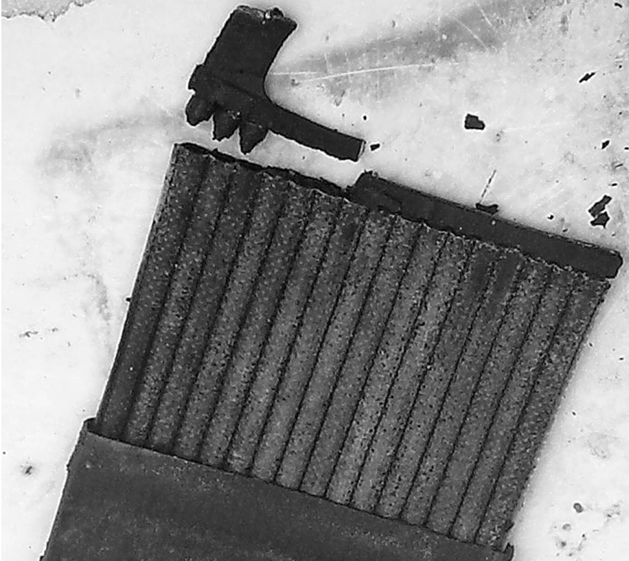
fig 41: positive plate corrosion
