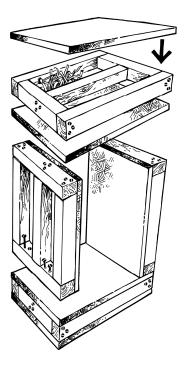
In some cases, the box frame can be attached to the wall plate, using that as a lintel instead of the box having its own top. In such cases, the settlement gap would be left at the bottom of the frame, not the top. However, this isn't a good option if the roof overhang would obscure any light coming in from the top of the window.
