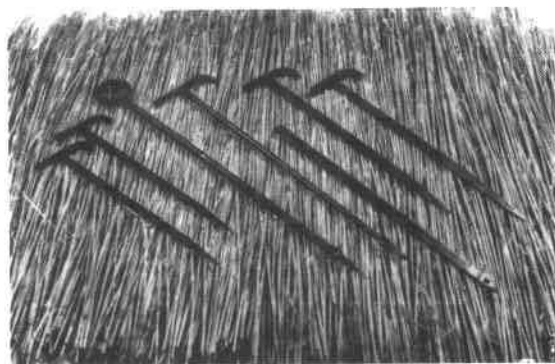
Shearing-hook used for cleaning down face of finished work.
