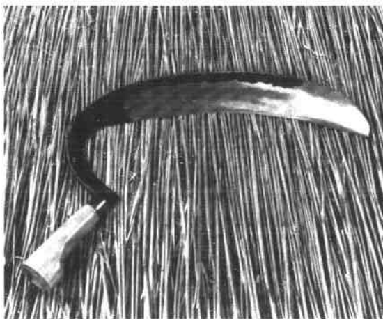
Shearing-hook used for cleaning down face of finished work.
