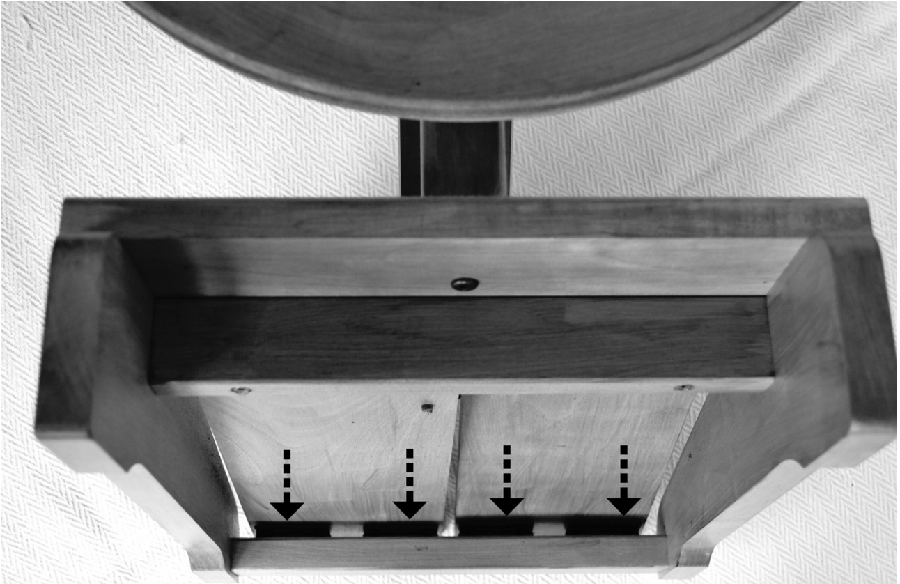
Treadle board from underneath showing oil points for metal hinges.
