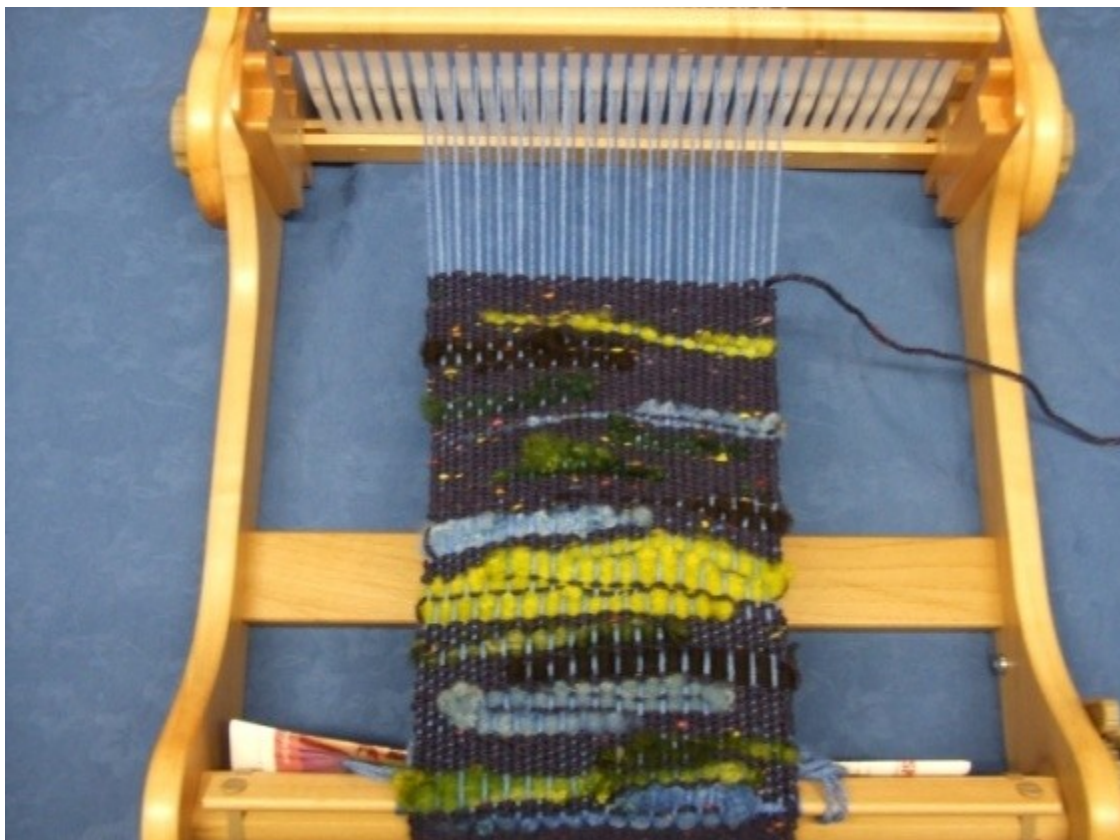
Ashford folding rigid heddle loom, called the 'Knitters' Loom', showing a 5 dent heddle in use.
