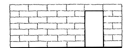
From accurate bale plans you can work out how many bales you need, as well as how many hazel stubs (two per bale on the first course), pins (two per bale for the fourth and sixth courses) staples (in every bale where it changes direction, e.g. corners) and other quantities of materials. Details of foundations, windows, first floor and roof can be worked out. You also now have the basis for drawing your own plans for planning permission.
