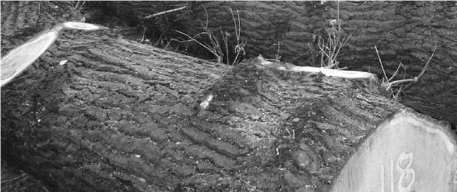
fig 29: oak log with large knot
