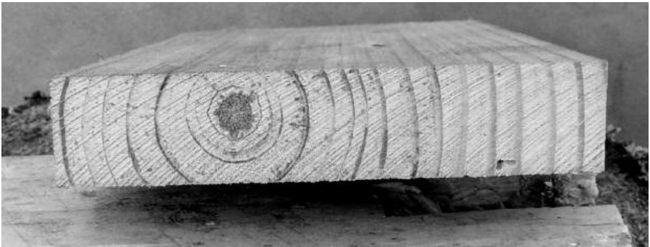
fig 4: early growth annual rings seen on the end of a softwood board
