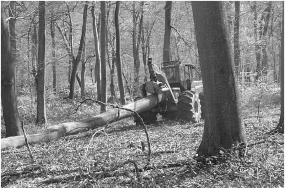
fig 86: skidder extracting whole poles
