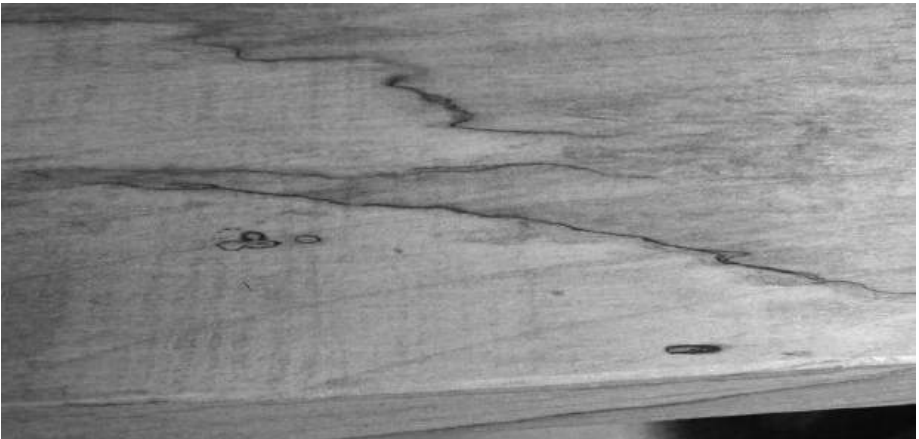
fig 26: spalting in a sycamore shelf
