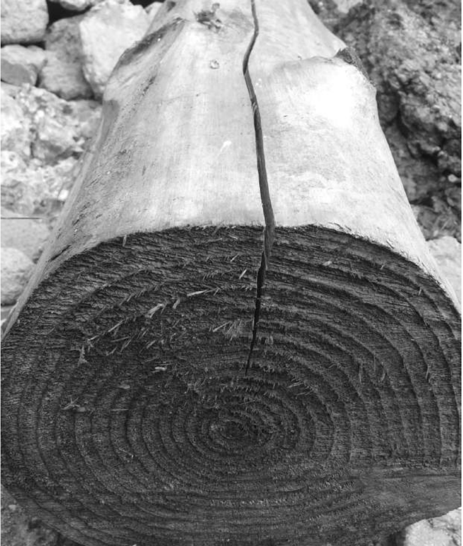
fig 76: drying shake in a red cedar log
