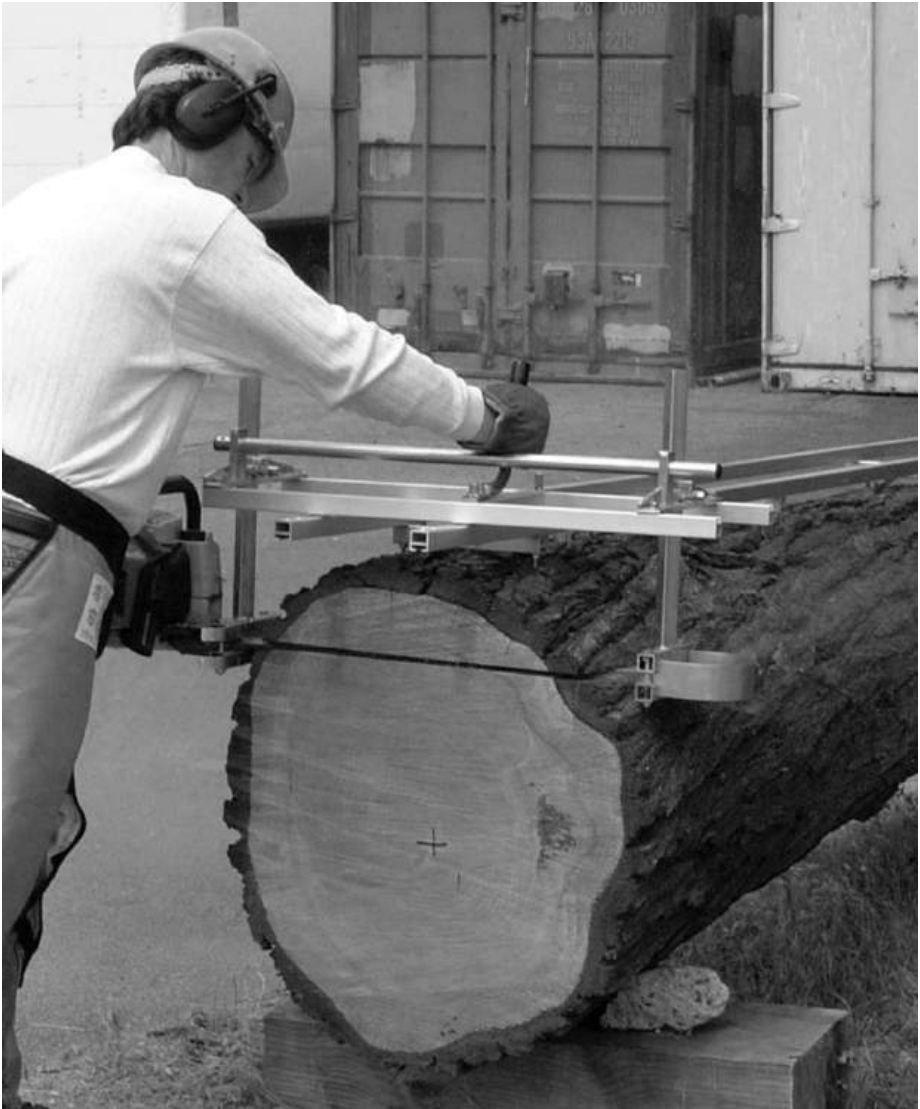
fig 45: first cut with an Alaskan mill
