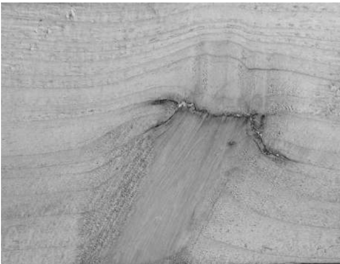
fig 12: grown over pruning cut
