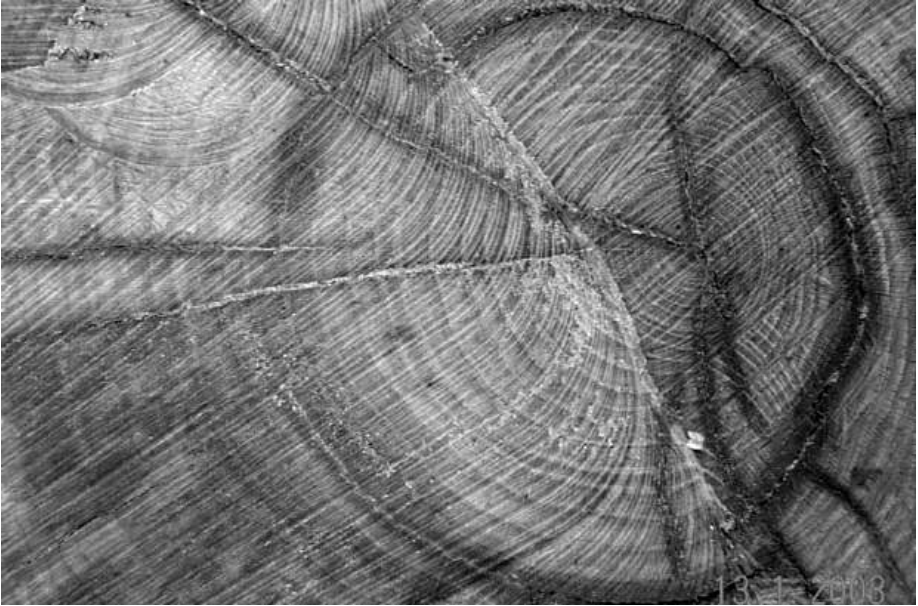
fig 22: star and ring shake
