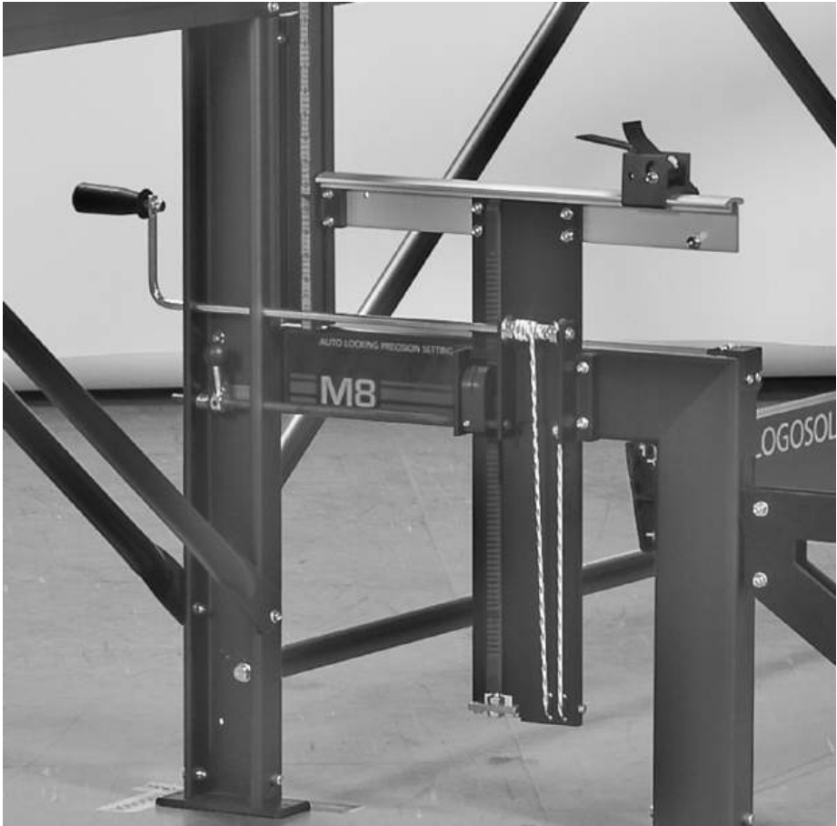
fig 50: log lift winch
