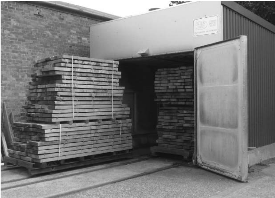
fig 80: loading a kiln
