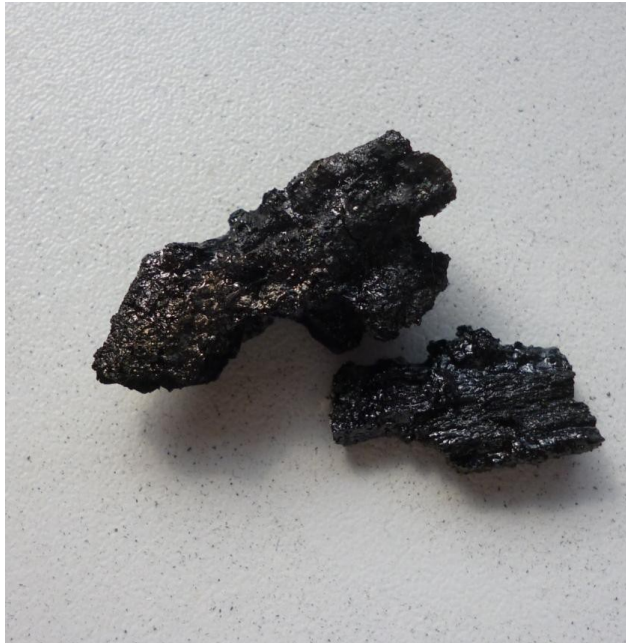
Fig. 18: fused deposit extracted from the combustion zone of a gasifier. Size = 2 cm across.
