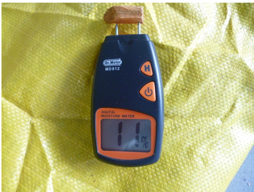
Fig. 16: determining the moisture content of wood chip
