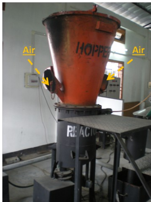
Fig. 6: Ankur downdraft gasifier showing two air inlets which take the air to the central section of the reactor
