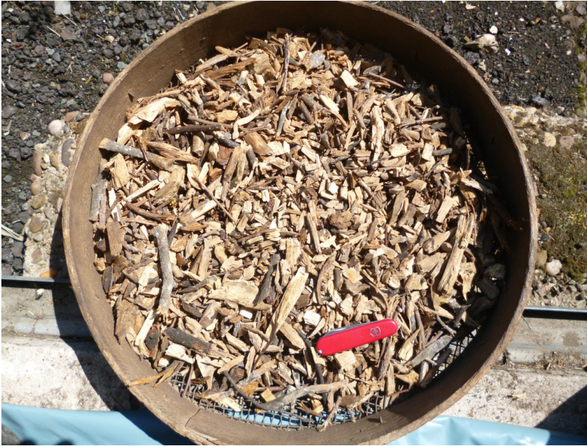
Fig. 14: wood chip from a drum chipper after screening with 1.2 cm sieve and fines removed. Note the large range in sizes. This is poor quality chip for a gasifier. It might be good for the mulch market, and it is the sort of stuff that you can get if you are not careful.
