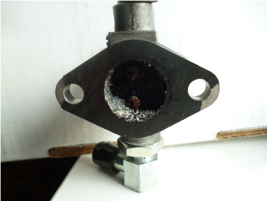
Fig. 23: tar and soot deposits in a producer gas engine throttle valve
