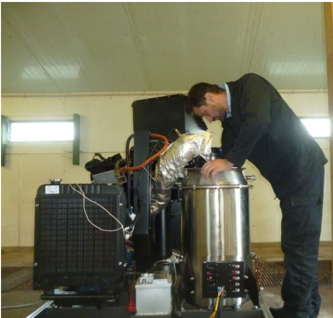
Fig. 5: re-connecting a thermocouple inside the reactor of a gasifier
