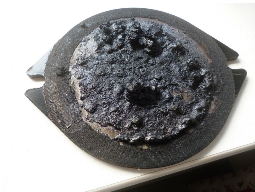
Fig. 29: solidified tar from a gasifier reactor top access cover. Diameter of item shown = 15 cm.
