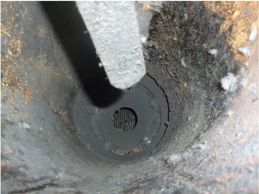
Fig. 8: looking from above into a gasifier reactor, the narrow “throat” section is discussed in The Downdraft Gasifier . The tongue-shaped protrubrance from the top middle is the auger paddle switch from the system shown in Figure 7. Ignore the blue fluffy deposits which came from my failed attempt to gasify recycled textile
