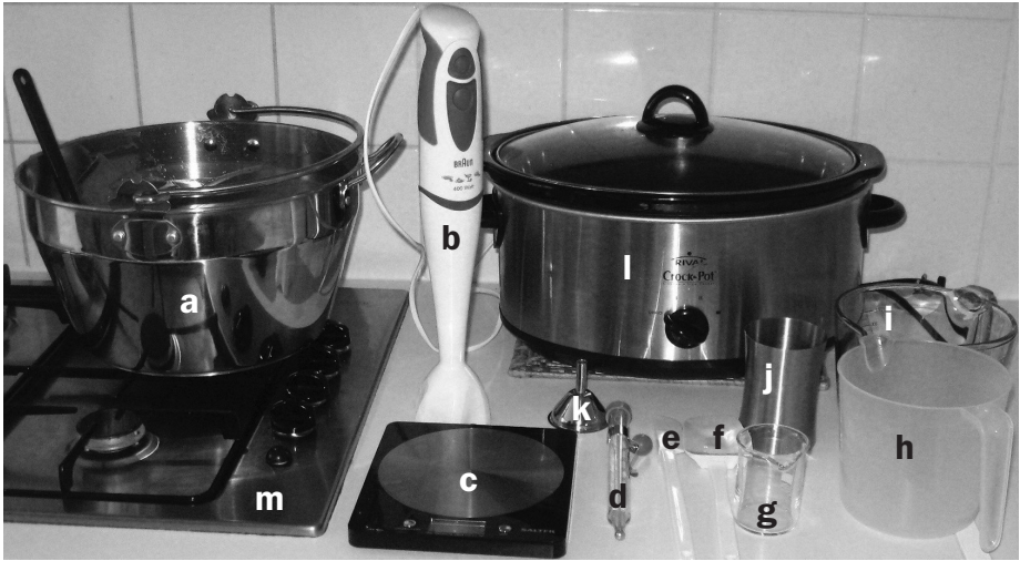
fig 5: basic equipment a) soap pot, b) hand blender, c) digital scale, d) thermometer, e) & f) spatulas, g) beaker, h) & i) measuring jugs, j) stainless steel container used to measure caustic soda, k) stainless steel funnel, l) slow cooker, m) stove
