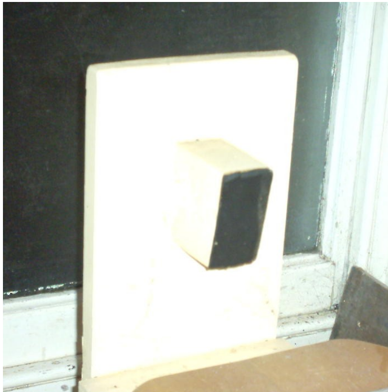
The lid-closer, positioned behind the toilet lid, allowing it to open to not quite vertical, and so it can't be left open.
