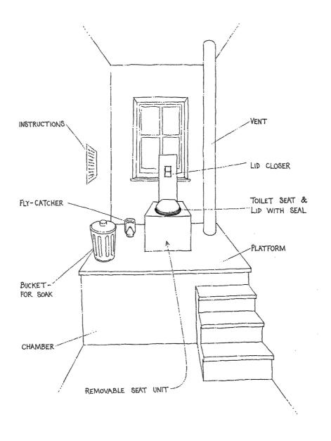
Components of a basic compost toilet (one chamber shown).
