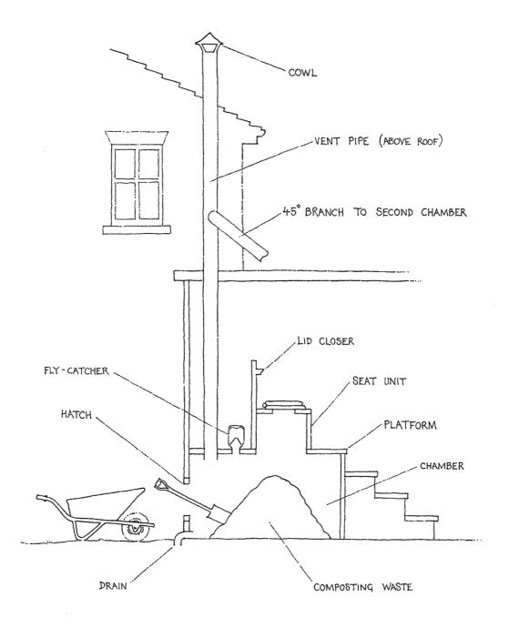
Cross-section of one chamber of a basic compost toilet.
