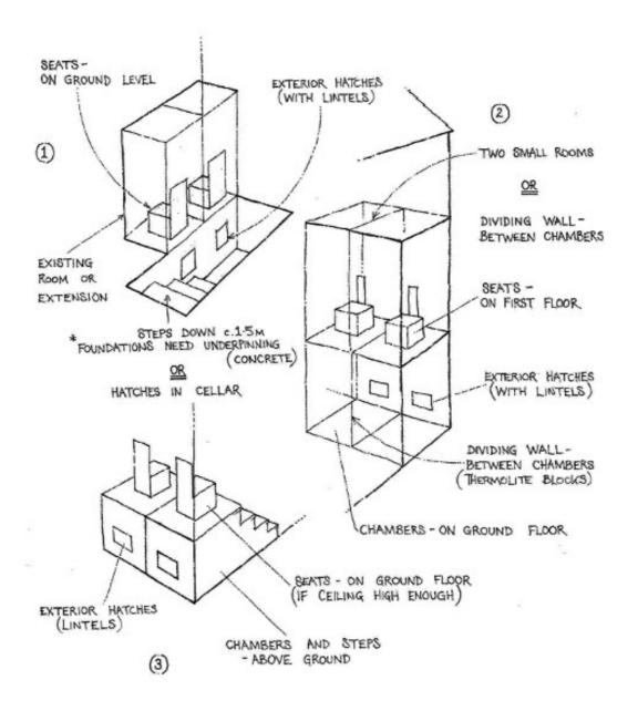
Various plans for locating compost toilets indoors; in no. 1, the steps will need a cover to prevent flooding. A better option might be to empty the chambers into the cellar.
