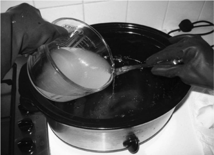
*fig 49: add the caustic solution to the heated fats and oils*
