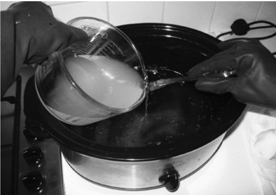
fig 41: add the caustic solution to the heated fats and oils
