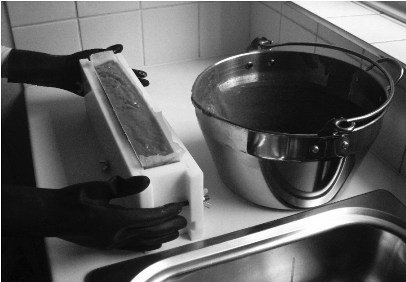
fig 22: level the mixture in the mould
