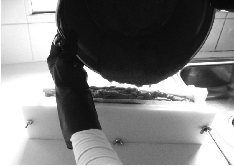
fig 21: pouring the mixture into the mould
