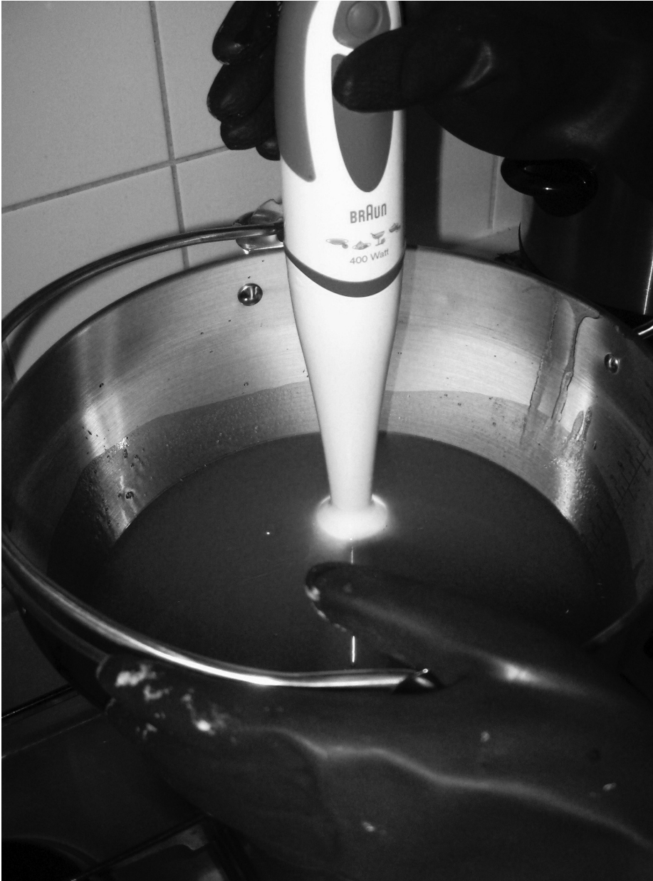
fig 16: bring the mixture to trace
