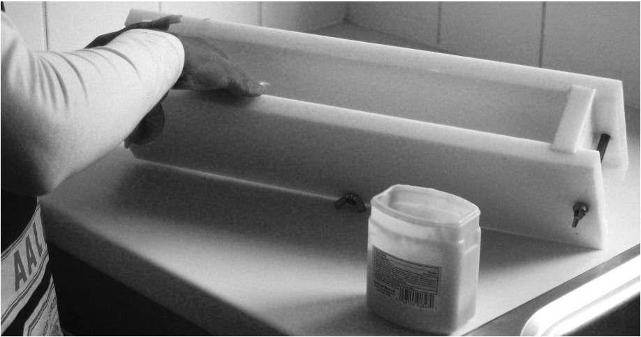
fig 9: grease all sides of the mould
