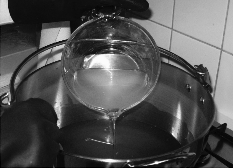
fig 14: add the caustic solution to the heated oil
