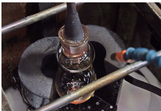
Blown glass being removed from the mould.
