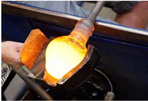
Shaping the gathered glass into a scoop before it's blown.
